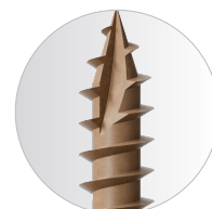
T-17 Tip Anti-friction point requires no pre-drilling
