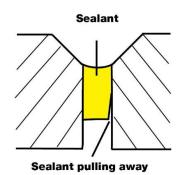
Wrong Sealant extends too deep into joint leading to tearing away from sides or splitting
